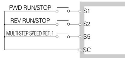
Note : When n004 is set to 0, 2, 3, 4, or 5, frequency reference 1 (n024) is disabled and frequency reference from volume (0) or control circuit terminal (FR, RP) is enabled.
