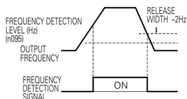
Frequency detection 2 (Output frequency  $\leq$  Frequency detection level)
