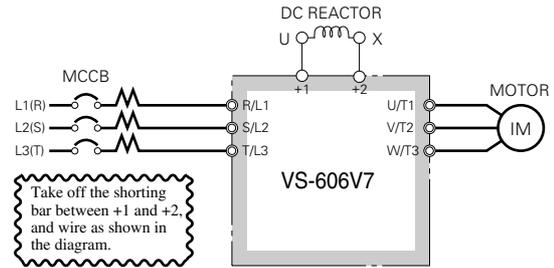
When power capacity is significantly greater when compared to inverter capacity, or when the power-factor needs to be improved, connect the AC or DC reactor.
