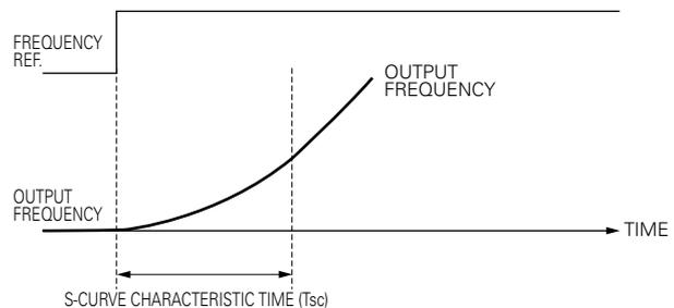
Time chart at FWD/REV run switching at deceleration to a stop
