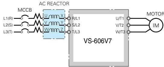
Be sure to connect AC reactor on inverter input side [L1 (R), L2 (S), L3 (T)].
