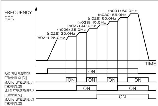
An example of 16-step speed change (9 to 16 steps) 16-step speed operation can be set by the following setting of multi-function input terminals (S4 to S7) with combination of 4 inputs in the same way as for 8-step speed operation.
