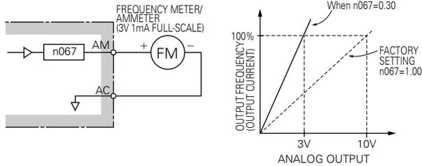
Set analog output voltage at 100% of output frequency (output current).
