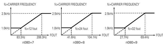
Carrier frequency initial value differs depending on inverter capacity as follows :
