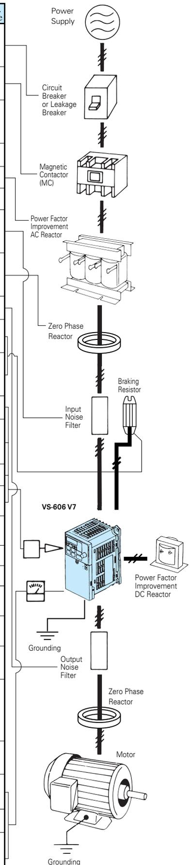
\*: When using a ground fault interrupter, select one not affected by high frequencies. To prevent malfunctions, the current should be 200mA or more and the operating time 0.1s or more.
