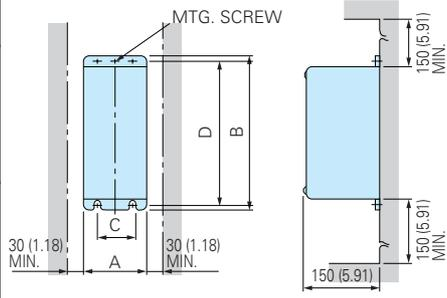
Braking Resistor [Dimensions in mm (inches)]
