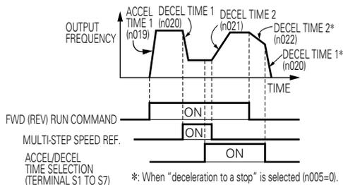
By setting input terminal function selection (one of n050 to n056) to "8" (accel/decel time select), accel/decel time is selected by turning ON/OFF the accel/decel time select (one terminal of S1 to S7).
