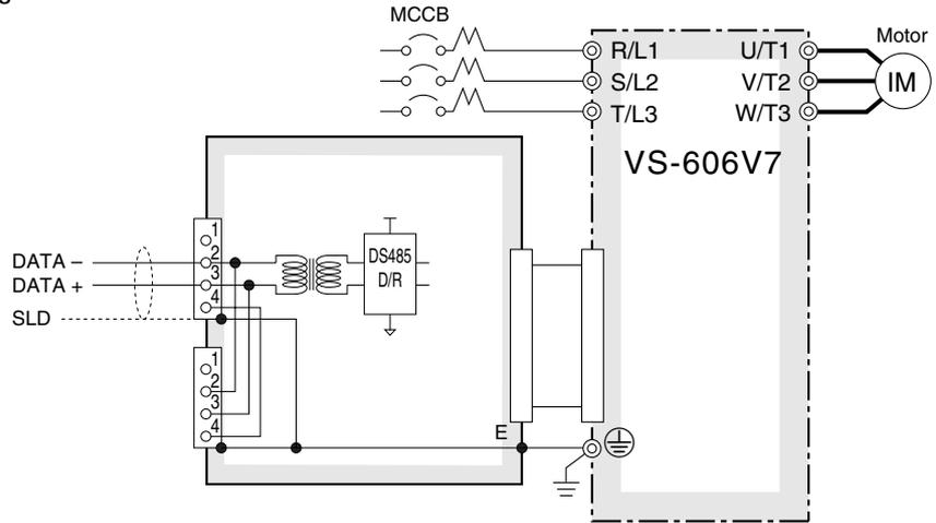
Note: Models of 3.7 kW or lower are currently available for MECHATROLINK communications. Requires the exclusive software for the SI-T/V7 installed in the inverter.
