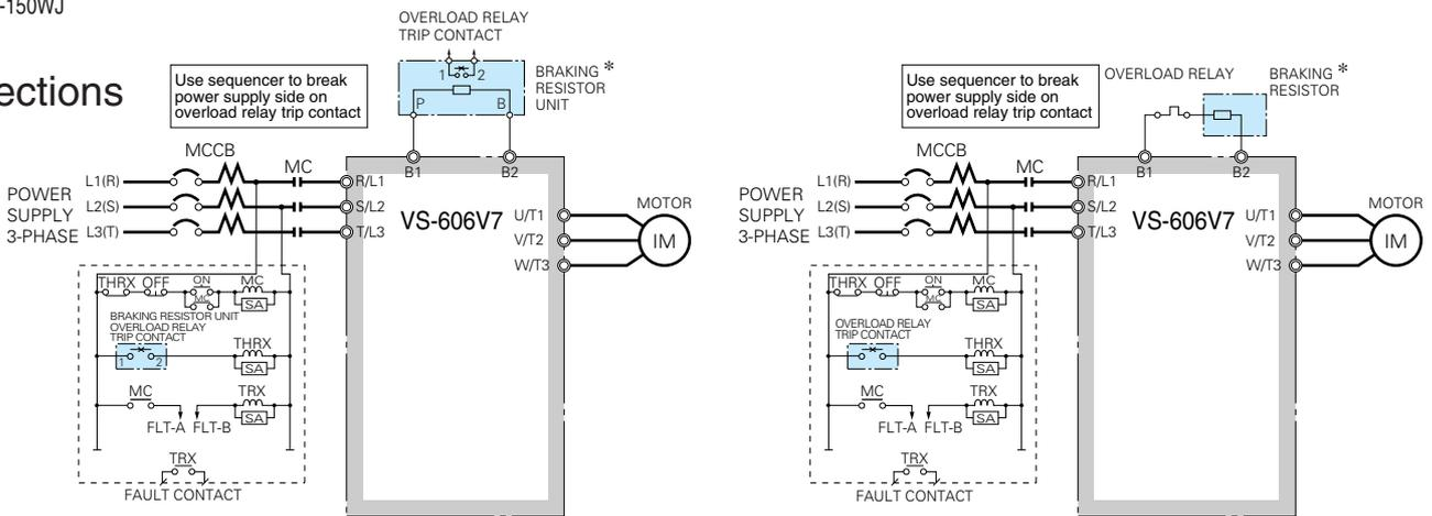
\* When using a braking resistor (option), set the stall prevention during deceleration to "Disabled" (n092=1) or the motor might not stop within the set deceleration time.
